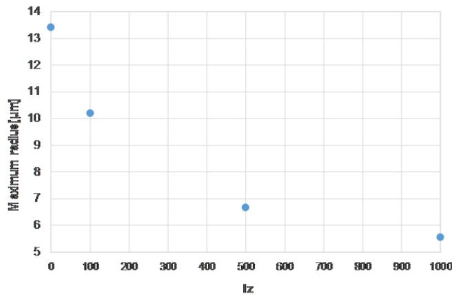
Fig. 5: Maximum mean radius in relation with different Zener parameters
