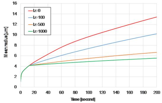
Fig. 4: Mean radius over time for three different values of Zener parameter
