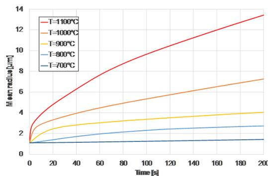
**Fig. 1: Mean radius over time for four different annealing temperature**
