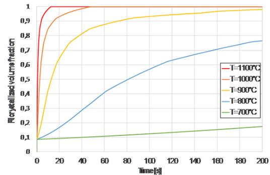
**Fig. 2: Recrystallized volume fraction over time for four different temperatures**
