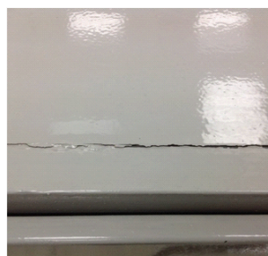
Fig. 3: A crack on the surface of the bench
