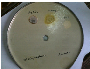
Fig. 2: The test conducted to check the bench paint
