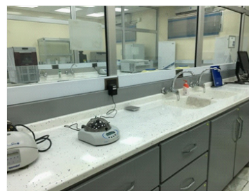
Fig. 10: The new benches with edges to control hazard of chemical spill
