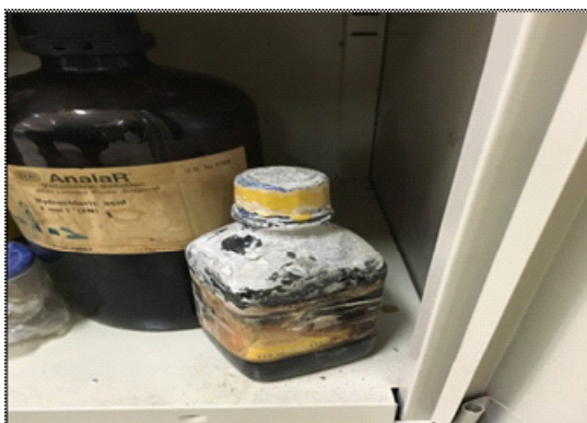
Fig. 18: Improper chemical storage
