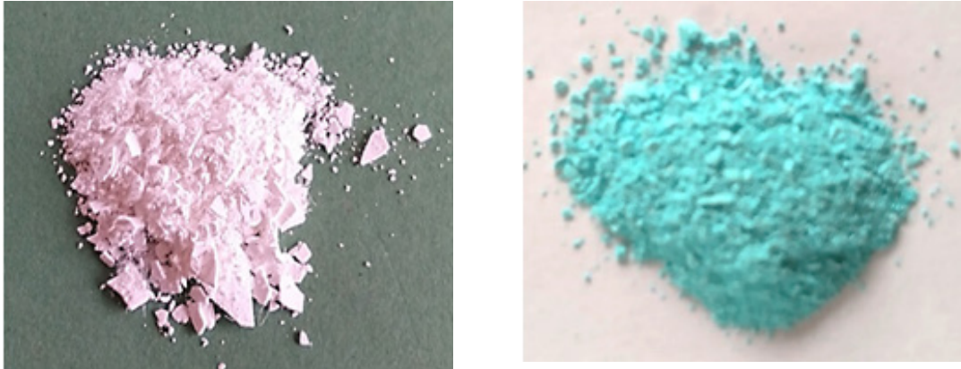
Fig. 1: The photos of the prepared MOFs (blue = Cu-OXA MOF and white = Zn-OXA MOF)
